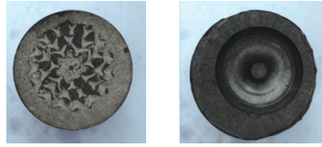
图1 牙轮钻头(左)、PDC钻头(右)可钻性实验样品 Fig. 1 Drillability test sample of cone bit(left) and PDC bit(right)
